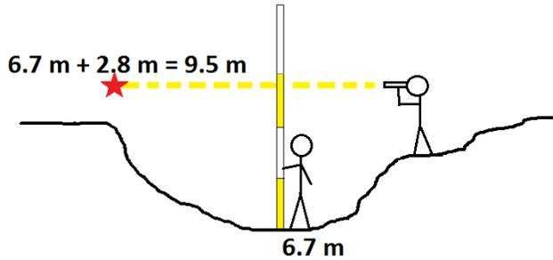
*Using the backsight and elevation of the point, the new height of instrument is calculated.*
