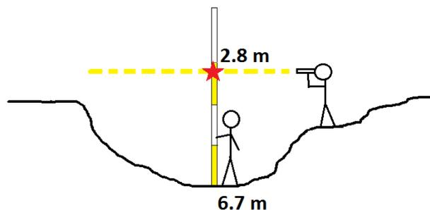
*The station is moved and a backsight taken to the pivot point.*
