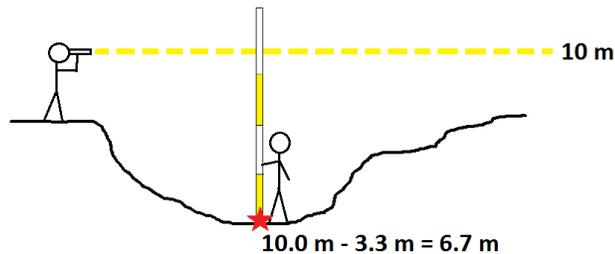
*Using the height of instrument and foresight, the ground elevation is calculated.*
