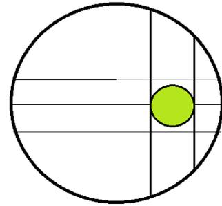
upper and lower stadia lines are used to gauge stadia distance, which is a method of reading distance off of the rod and level alone (based on parallax). We won't need to do this in lab, but for future reference, if you take the readings at the upper and lower stadia lines, subtract them, and multiply by 100, that is the distance in meters between the level and the stadia rod. The bubble needs to be lined up with the middle stadia line in order to be level.
