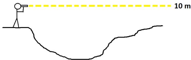
*The eye height of the leveler forms the height of instrument – in this case set to an arbitrary 10 m to avoid negatives.*
