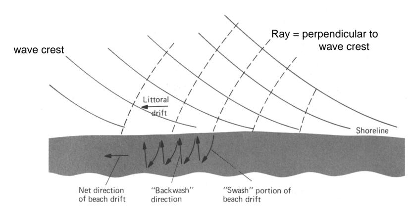
In shallow water, wave speed decreases as water depth decreases waves travel progressively slower as depth decreases, therefore crests bend = wave refraction
