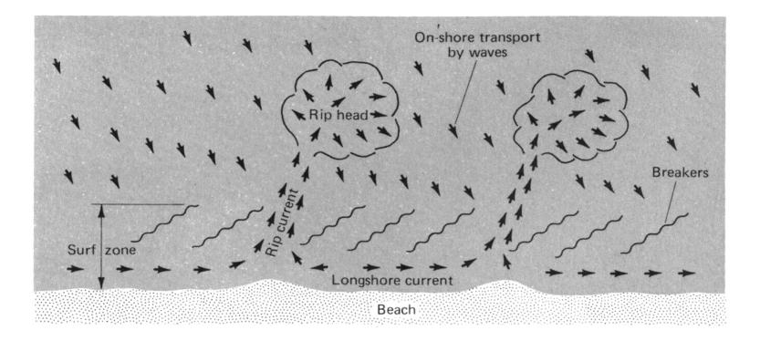
Rip currents are the primary mechanism for returning water through surf zone, and are the most dangerous for swimmers Also broad, weak flow near seabed = undertow
