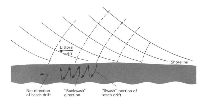
Waves break at angle to shore, which causes swash at angle to shore Backwash follows gravity down foreshore Net effect is water and sediment transport along shore
