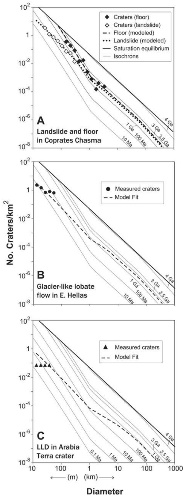
**Figure 3.** Model fits to prior studies using crater-frequency distributions to date small deposits, assuming a mixed population of primary and secondary craters. Crater counts from (a) Quantin *et al.* [2004] and (b and c) Hartmann [2005]. Isochrons and saturation equilibrium line from Hartmann [2005].
