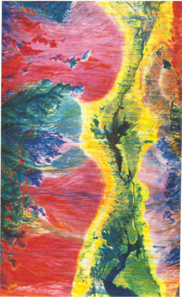
Figure 2. Three enhanced versions of a TIR image of Death Valley, California, acquired by NASA's TIMS scanner near noon on 27 August 1982. TIMS acquires data in six bands centered at wavelengths 8.3 \mu\text{m} , 8.7 \mu\text{m} , 9.1 \mu\text{m} , 9.8 \mu\text{m} , 10.4 \mu\text{m} , and 11.3 \mu\text{m} (Palluconi and Meeks, 1985). North is up, the image is \sim 25 \text{ km} from top to bottom. The nadir ground pixel size is \sim 18 \text{ m} . The data were nominally calibrated, scan by scan, using dual on-board blackbody measurements, and geometrically resampled to rectify scan-angle foreshortening. Both the above corrections were done at the Jet Propulsion Laboratory. a) Standard false-color composite, with R , G , and B = Channels 5, 3, and 1, enhanced by stretching radiance data only; b) color ratio composite, with R , G , and B = Channels 5/4, 3/4, and 1/4; c) decorrelation-stretched image, with R , G , and B = Channels 5, 3, and 1 (JPL Photo # P-26340).
