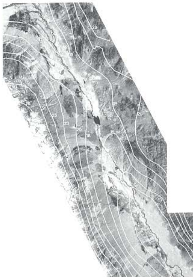
Figure 6. Image showing mean annual precipitation (MAP) isohyetal lines (Hollet et al., 1988) superposed on an "inverted" shade fraction image (Part I). Numbers on isohyets are cm. MAP data were not available for the entire study area [Fig. 1a]. The minimum MAP is displaced eastward from the center of Owens Valley, because of the rain shadow of the Sierra Nevada. Isohyetal lines are elevation-transgressive, with rainfall at constant elevation generally increasing northwards.
